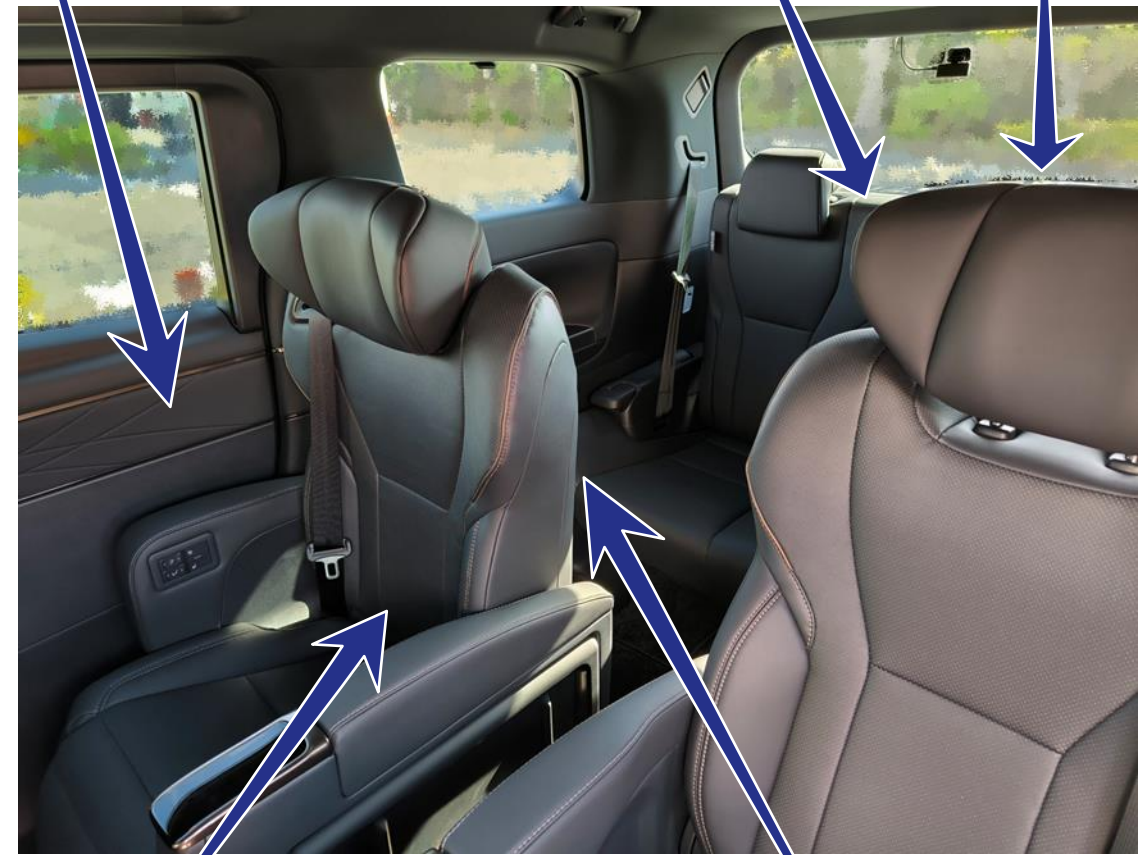
Seat backboard: TPO composite and PVC composite
